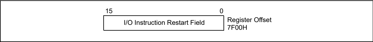
Figure 34-5. I/O Instruction Restart Field
